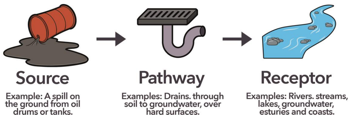
Figure 2: Example of a pollution linkage using the source > pathway > receptor model.
