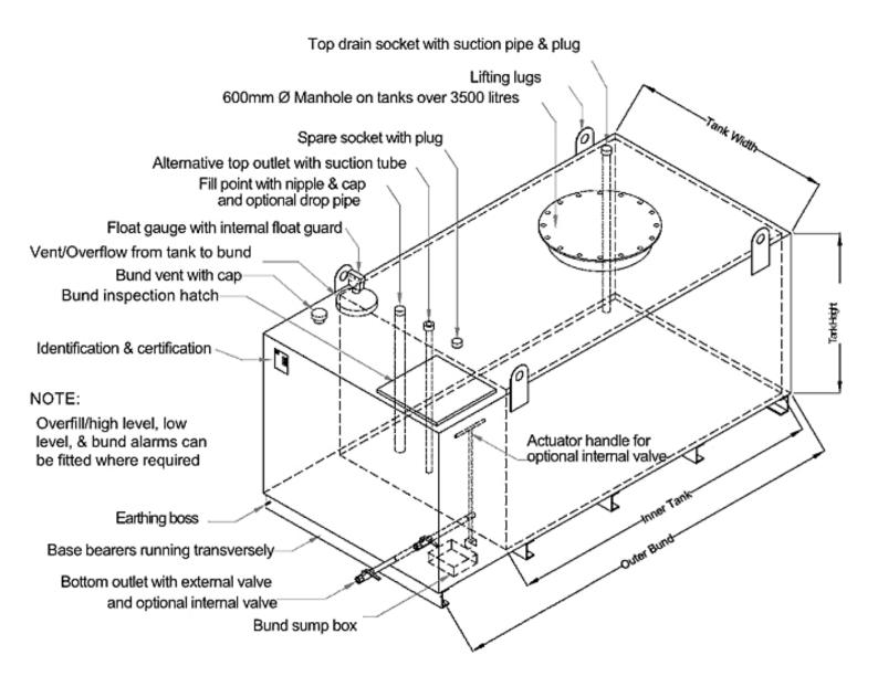
**Figure 2. Example of integrally bunded tank** (could be constructed of metal or polyethylene and may not be this shape and design)
