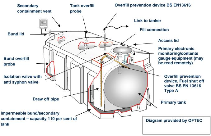
Figures 1 and 2 are for illustration only. Different configurations exist depending on the manufacturer, type of tank and installation. We normally recommend top tank outlets, as manual valves on bottom tank outlets must have someone in attendance.
