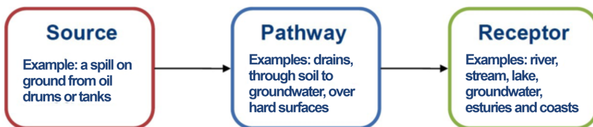
Figure 1: Example of a pollution linkage using the source > pathway > receptor model. NOTE: Groundwater is both a pathway and a receptor.
