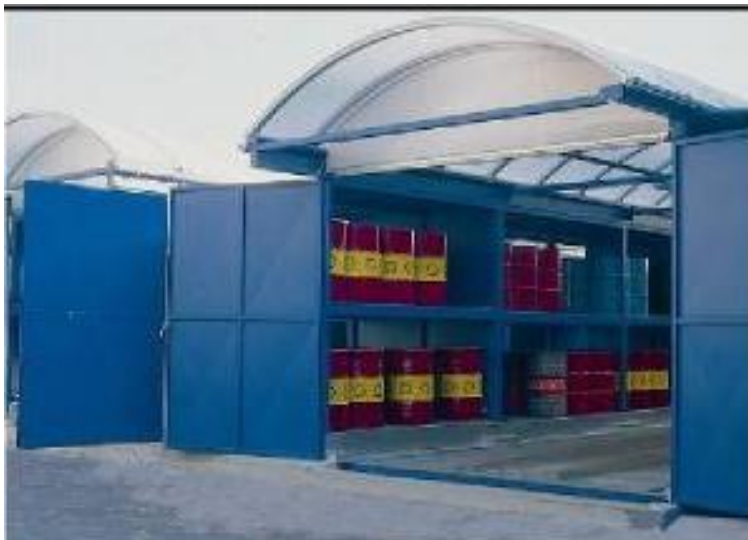
Figure 3: Safe storage, bunded and under cover
