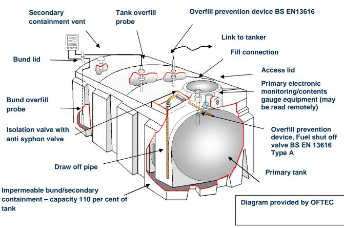
Figures 1 and 2 are for illustration only. Different configurations exist depending on the manufacturer, type of tank and installation. We normally recommend top tank outlets, as manual valves on bottom tank outlets must have someone in attendance.
