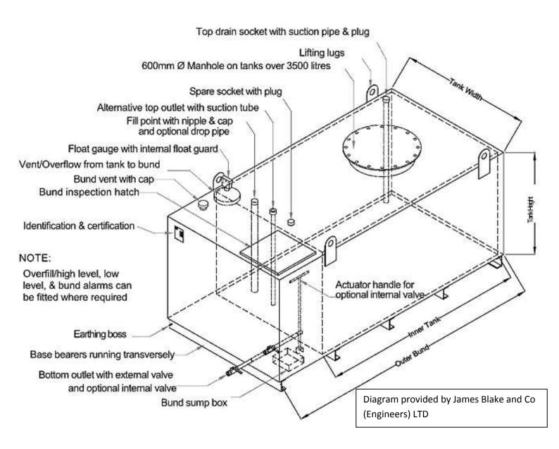
**Figure 2. Example of integrally bunded tank** (could be constructed of metal or polyethylene and may not be this shape and design)
